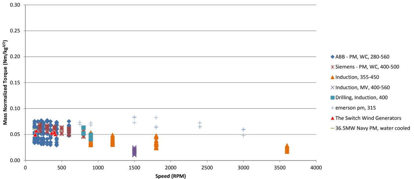
Fig. 2 – Mass Normalized Torque (MNT) vs speed on production motors and generators
