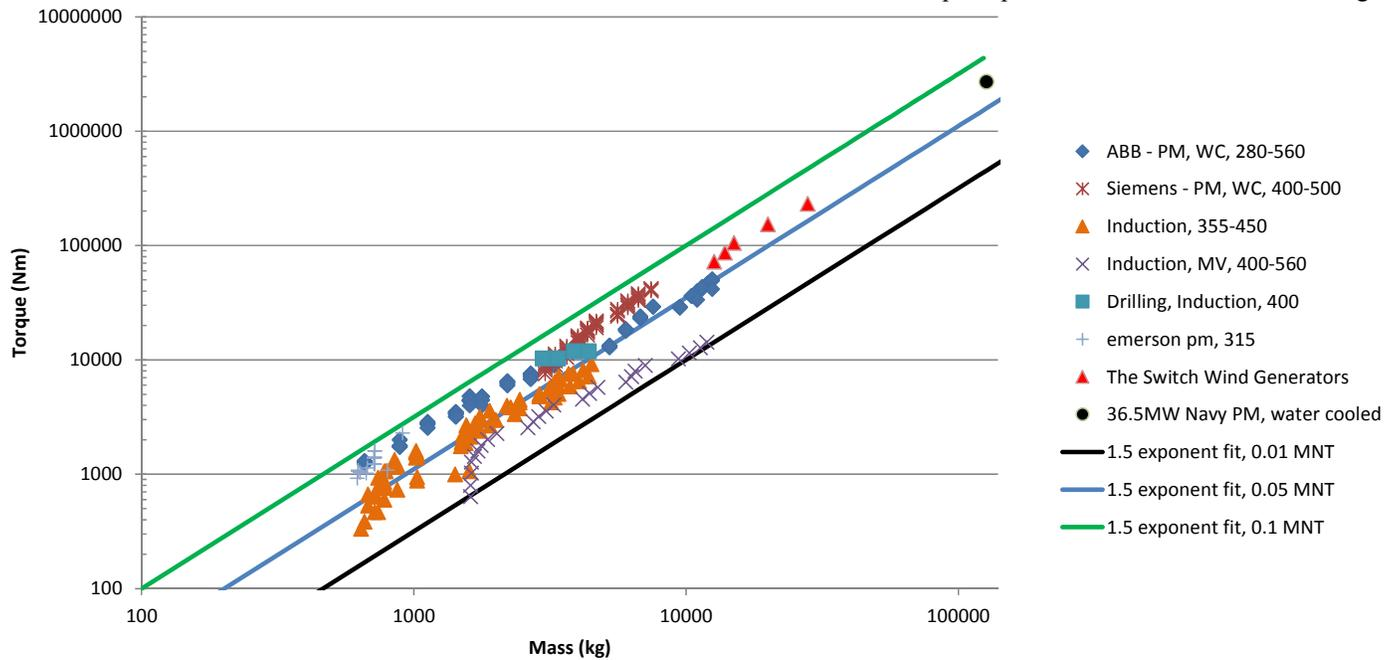
Fig. 1 – Torque vs Mass of Commercial Motors
